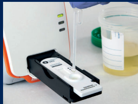
Insert CLINITEST hCG pregnancy test cassette and pipett sample.
